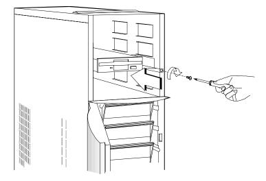
Figure 3-10. Securing the Drive
